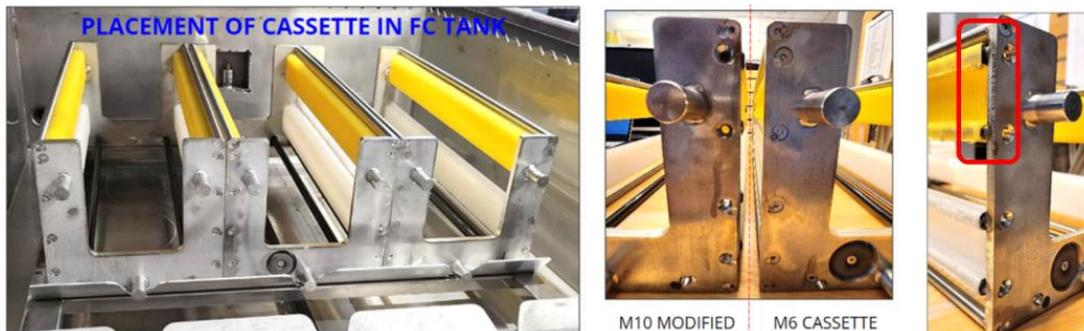
Figure 10: Placement of three cassettes side-by-side in the final cleaning (FC) line tank (left), comparison of the modified M10 and M6 cassettes (middle), and close up of the frame plate extending beyond the frame of the modified M10 cassette (right).
