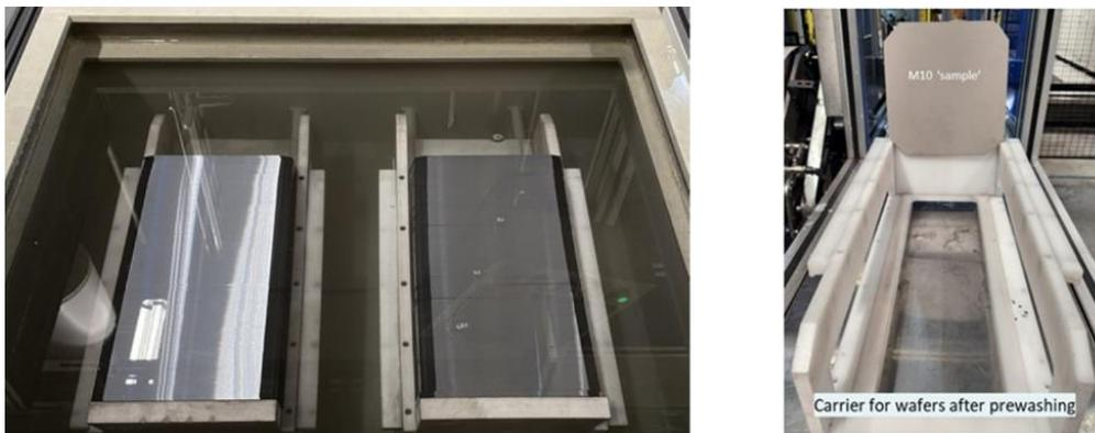
Figure 7: Singulation wafer carriers filled with M6 wafers (left) and comparison of existing carrier with M10 wafer size indicating the need for width adjustment
