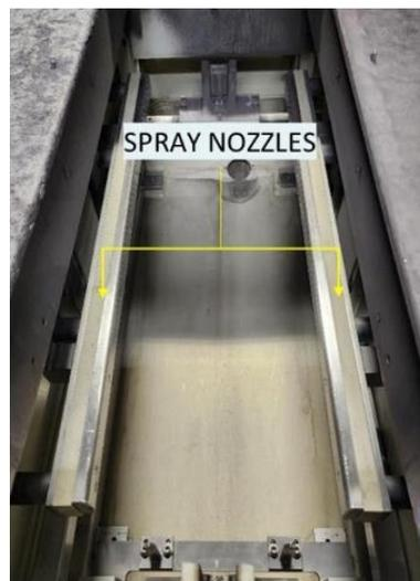
Figure 6: Picture of the spray nozzles of the prewash equipment
