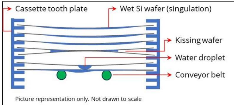
Figure 12: Schematic drawing of potential kissing wafer phenomenon during cassette loading.
