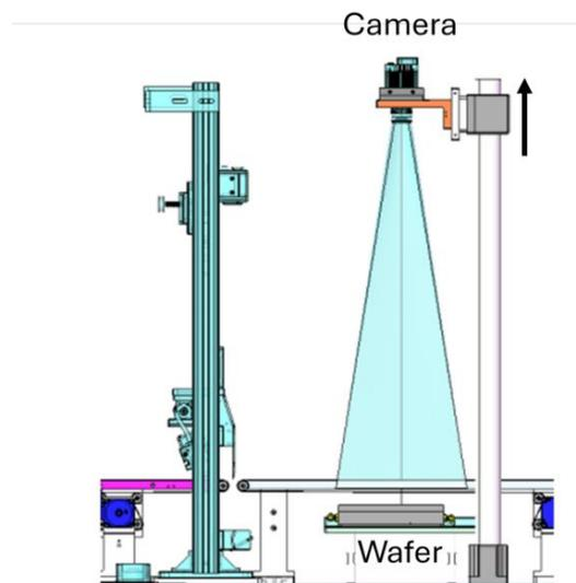
Figure 18: Schematic drawing of set-up for wafer geometry measurements. The camera position needs to be adjusted to capture the increased wafer area.
