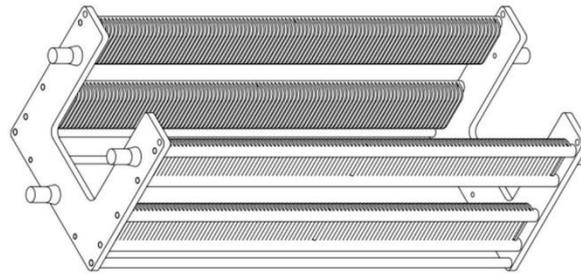
Figure 9: Generic design of wafer cassette for batch-wise cleaning
