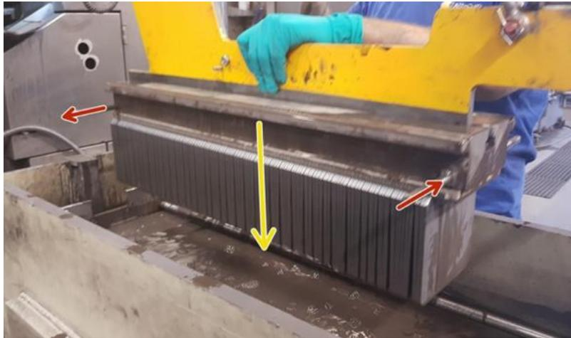
*Figure 3: After slicing the block will be unloaded from the wafer saw and lowered (yellow arrow) into a transfer cart filled with cutting fluid or process water.*
