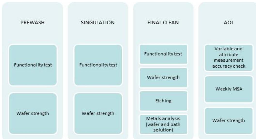
Figure 20: Overview of tests and verifications for the M10 modifications of the wafer line
