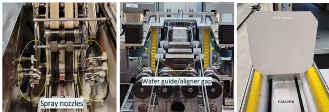
Figure 8: Images of spray nozzle positioning during wafer separation (left), wafer position aligner (middle), and comparison of M10 wafer size with M6 wafer cassette.
