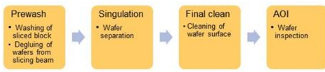
*Figure 4: Wafer cleaning process steps: (i) Prewash, (ii) singulation, (iii) final cleaning, and (iv) automatic optical inspection (AOI)*
