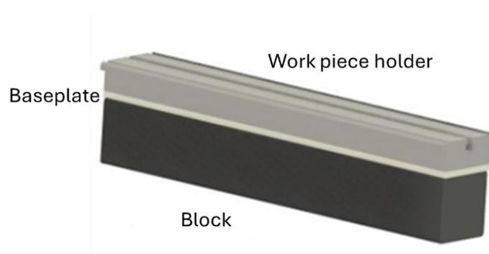
Figure 2: Schematic drawing of the slicing assembly: Monocrystalline silicon block glued on a baseplate, which is glued on a work piece holder
