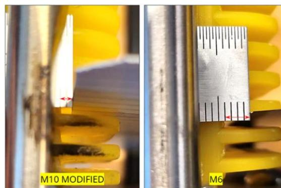
Figure 11: Comparison of the dimensional tolerance of the wafer edges for the modified M10 (left) and the original M6 (right) cassettes
