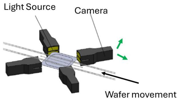
Figure 19: Schematic drawing side chip detection (adapted from Applied Materials)
