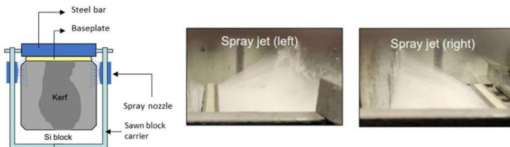
Figure 5: Schematic drawing of water spray nozzles during prewash (left) and spray jets during operation (middle and right)
