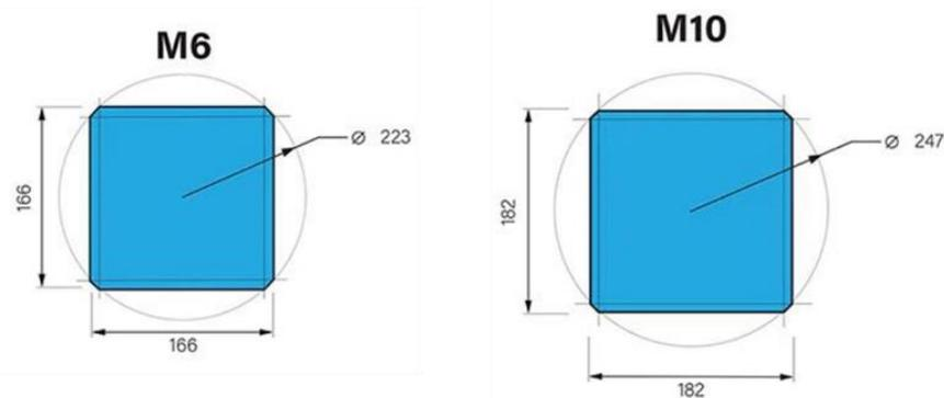
Figure 1: Comparison of M6 and M10 wafer formats (dimensions in mm).
