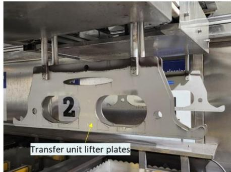
Figure 14: Image of the transfer unit lifter plates of the final cleaning line
