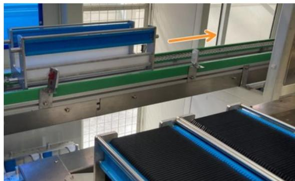
Figure 16: Return belt for transfer of wafer cassettes from unloading to loading
