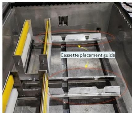
Figure 15: Image of the cassette placement guides inside the tanks of the final cleaning unit
